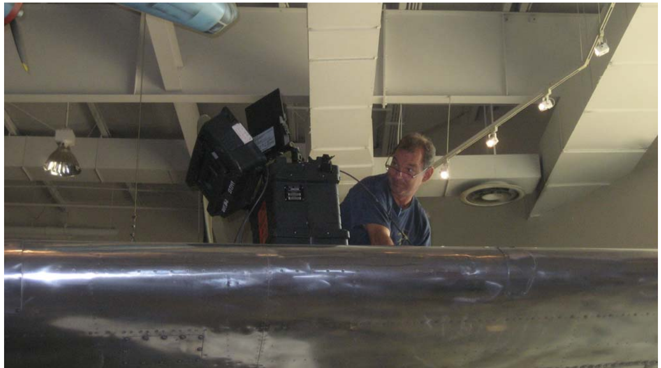
Jim checking a fuel tank while watching the boroscope's screen
