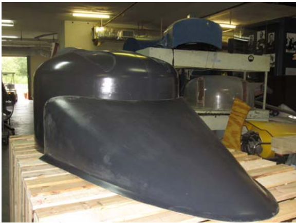
Chin turret cap and fairing – front and rear. Photos by Bill Burkel
