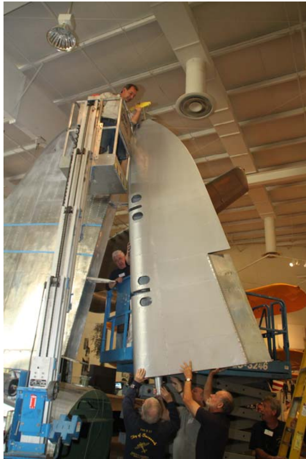
Mounting the newly refurbished rudder, thanks to LMI Corporation.
