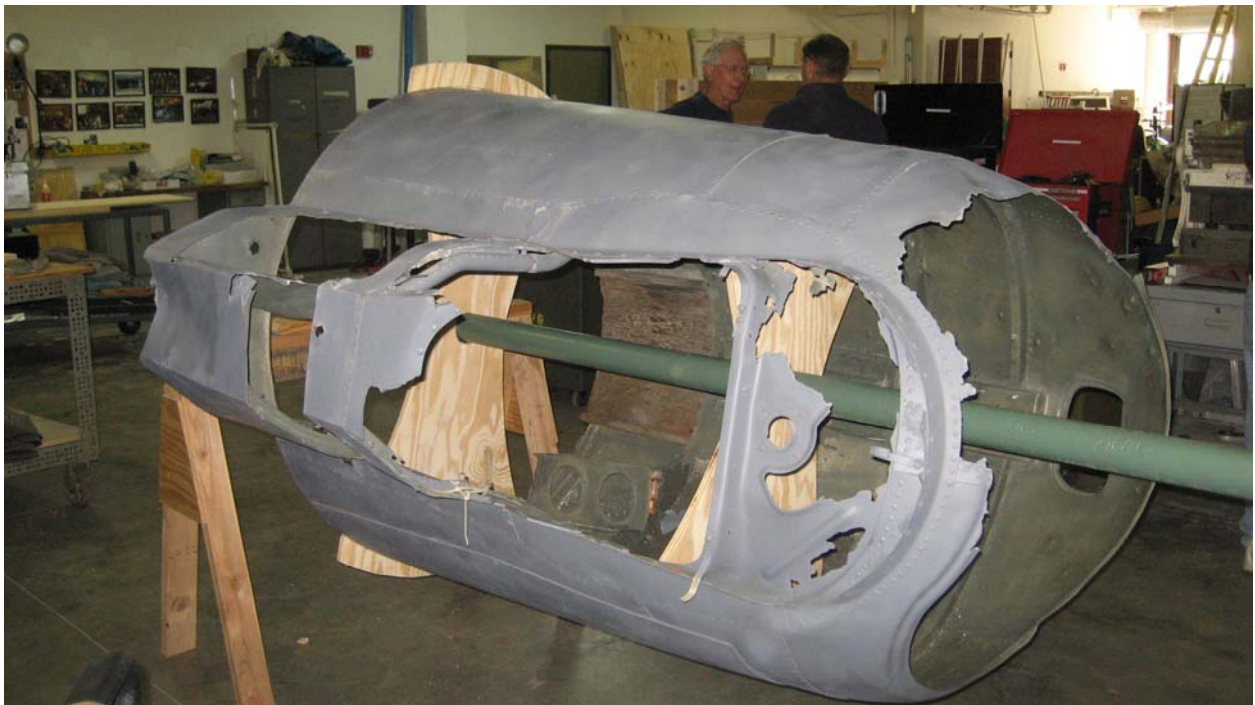
Gil Patrick's famous invention, designed to hold the tail turret during restoration
