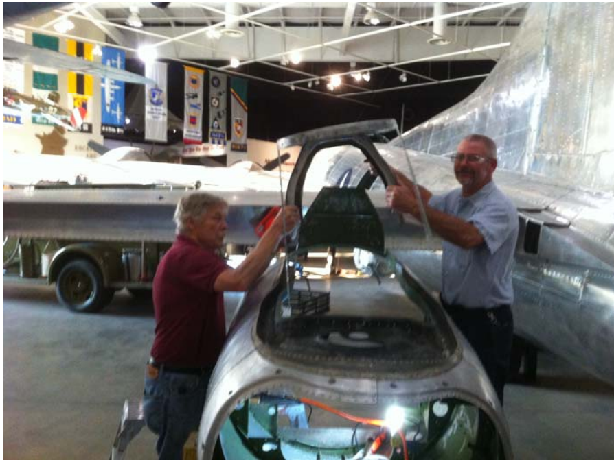
Jack Nilsen and Jim Odom removing the greenhouse structure from the Grissom AFB Cheyenne turret on loan to the City of Savannah
