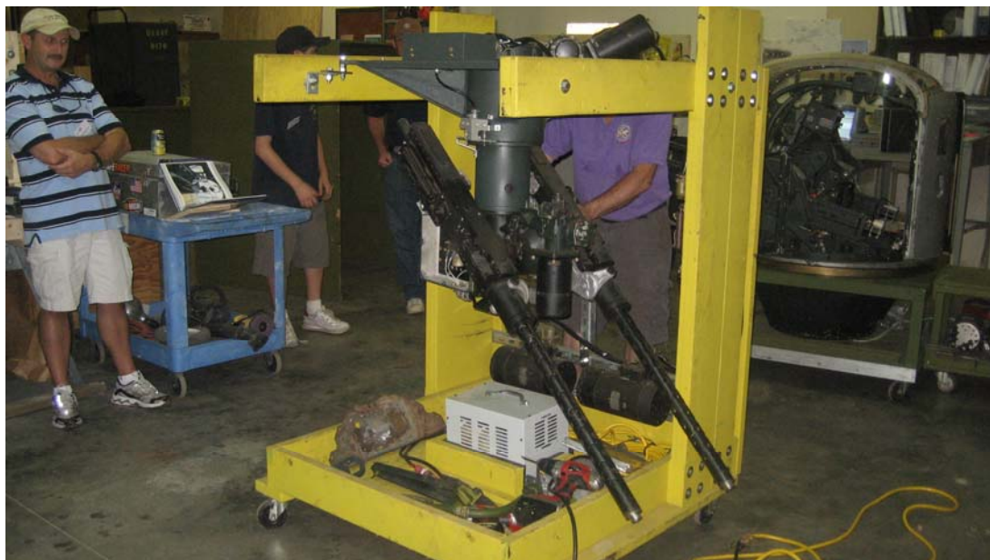
Fred Beiser’s B-17 nose turret on its demonstration stand.
