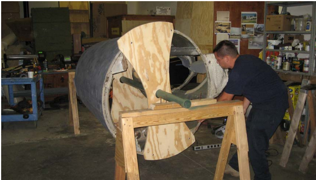
John Finch checking out Gil Patrick's "rotisserie" mounting device for the tail turret.
