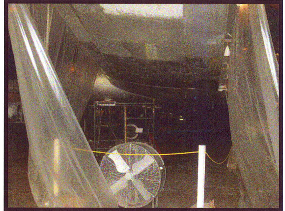
Hopefully the ColdJet will aid in the tedious job of cleaning the undersides of the wings
