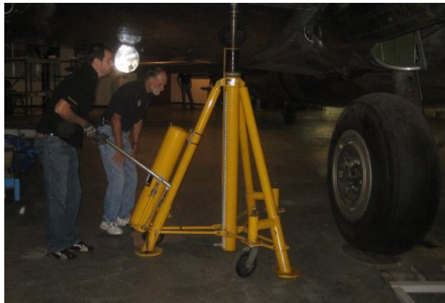
AAS employee John Miller and Danny Harden, Wednesday Crew Chief on the " City of Savannah ", working the jack to lower " City " onto the stanchions that will support the aircraft on the floor of the Mighty Eighth's Combat Gallery.
